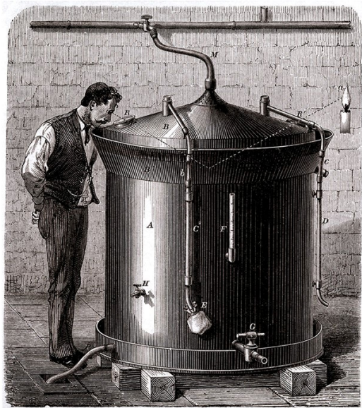
Engraving of a beer vat designed by Louis Pasteur, ca. 1880 Courtesy National Library of Medicine. The closed fermentation tank prevented air-borne bacteria from entering and spoiling the brew.
