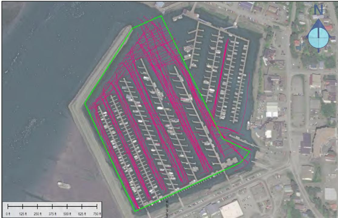
Figure 9 Sub-bottom Profiler Survey Lines
