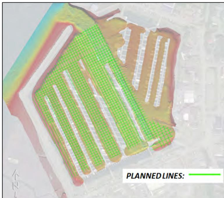
**Figure 8 Planned Survey Lines spaced at 25ft (Overview)**
