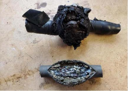
Corroded wire and splice from G Float
