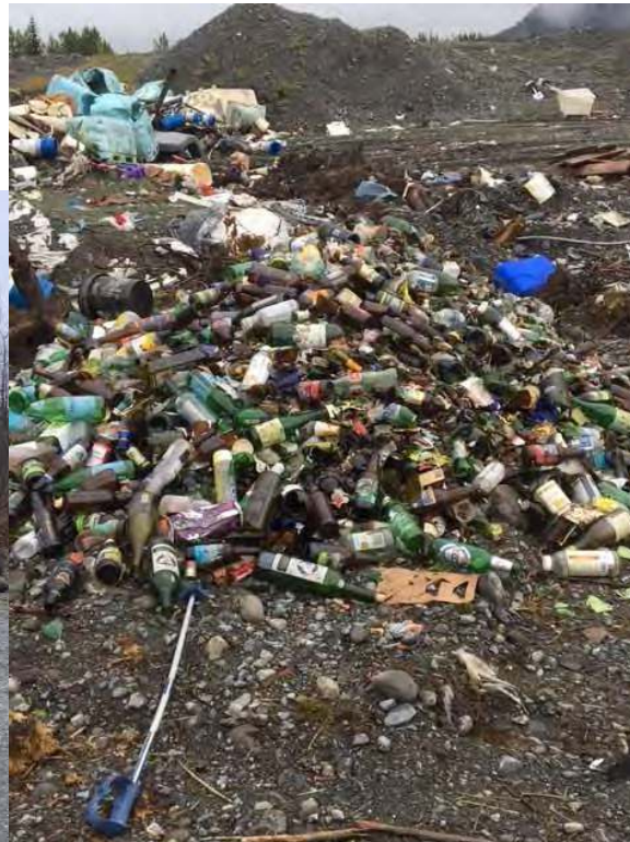
Glass to be crushed and used for daily cover
