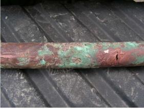
Photo on left is a close up of the hole and the photo on the right shows the overall condition for 4" of pipe. This is how it probably looks for all 150' from the residence to the main. A 3' section was replaced during this repair.
