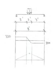
W= 144 PSF MAX UNIFORM LOAD > 100psf Ground Snow load for Cordova
