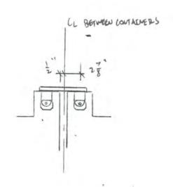
I PLATE WORKS TO TRANSFEL WIGHT, CHECK CONTAINER WT TO RESIST WOLFT I CONTAINER WT = 8600 Myz = 4300 M > 2606 M UPLETT
